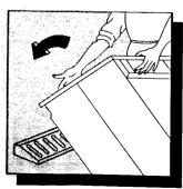
Remove the polystyrene block from the bottom of the machine.
